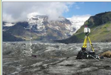
Fig. 1.1 TLS and wind tower on rock covered ice surface, Svinafellsjökull glacier, Iceland.
